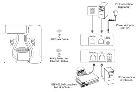
**Note:** PoE is only applicable to the SIP-T19P IP phone. If inline power (PoE) is provided, you don't need to connect the power adapter. Make sure the Etherne cable and hub/switch are PoE compliant.
