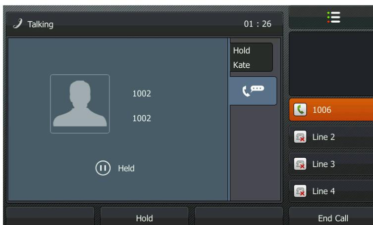
If multiple calls are placed on hold on more than one line keys, you can view the details of the call by tapping the corresponding line key, and then press the **Resume** soft key to retrieve the call.
