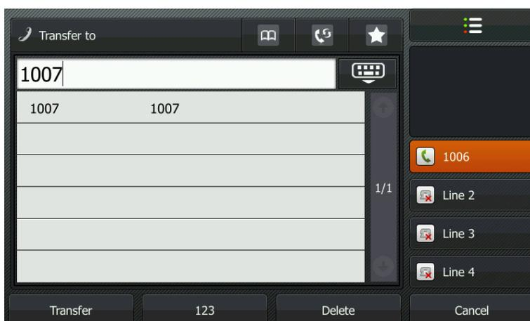
3. Press **Transfer** or the **Transfer** soft key to complete the transfer.
