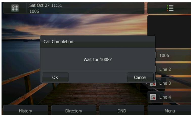
1. Tap the **OK** soft key, the phone returns to the idle screen and call completion is activated.
